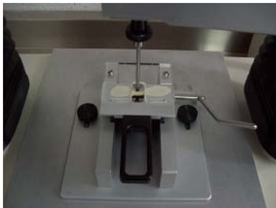
Figura 9. Aditamento Kieffer Dough and Gluten Extensibility Rig
