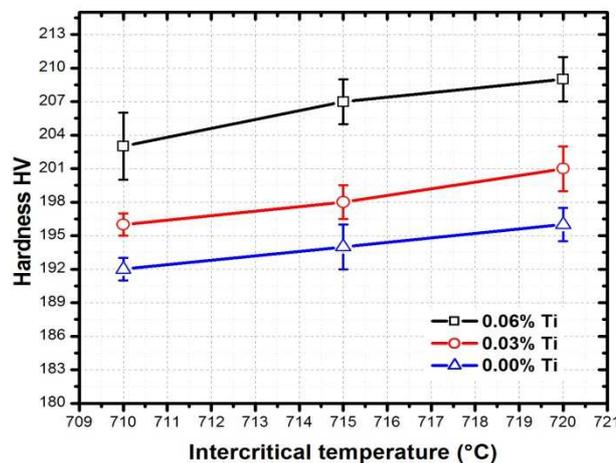
Fig. 5 Hardness (HV) results of the DP steels
