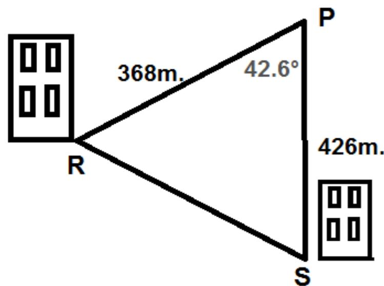
$$\begin{aligned} P &= 42.6^\circ & p &= 293.44\text{m.} \\ r &= 426\text{ m.} \\ s &= 368\text{ m.} \end{aligned}$$
