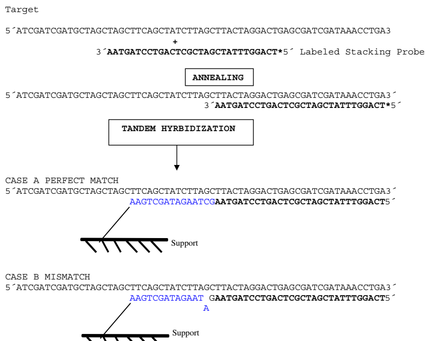
Fig. 2 Strategy for detection of point mutations by tandem hybridization. (A) The DNA target should be first annealed with a labeled stacking probe. The partially duplexed target is then hybridized to a specific short capture probe that is covalently attached to the surface of the sensor. The capture probe is designed to hybridize to the target DNA in tandem or contiguously with the longer stacking probe. Base
