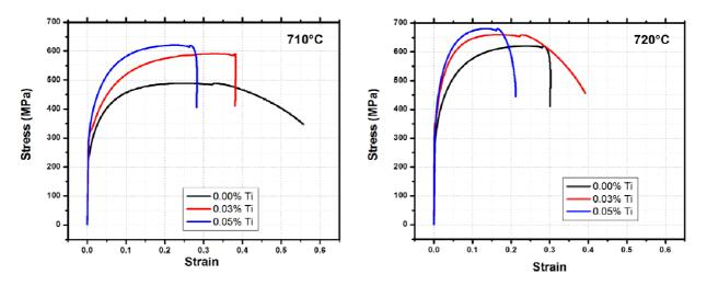
Fig. 6 Stress - strain curves for the DP steels
