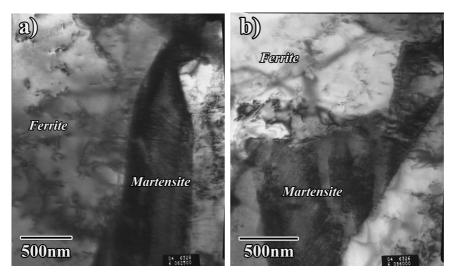
Fig. 4 TEM micrographs of the 720°C treated steel containing 0.06% Ti
