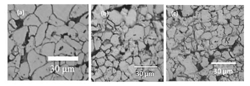
Fig. 2 Pearlite islands formed in the center of the ferrite grains, a) base DP1 steel, b) 0.03% Ti DP2 steel, and c) 0,05% Ti DP3 steel.
