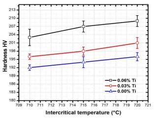
Fig. 5 Hardness (HV) results of the DP steels
