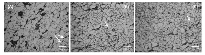
**Fig. 1** Optical microscopy of the DP steels after the thermomechanical treatment: (a) base DP1 steel, (b) 0.03% Ti DP2 steel, and (c) 0.05% Ti DP3 steel.
