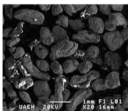
Figure 1 E-waste powder micrograph at 20X using 20 kV.
