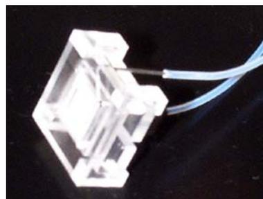
**Fig. 3** Photograph of chamber used for flow-through hybridization
