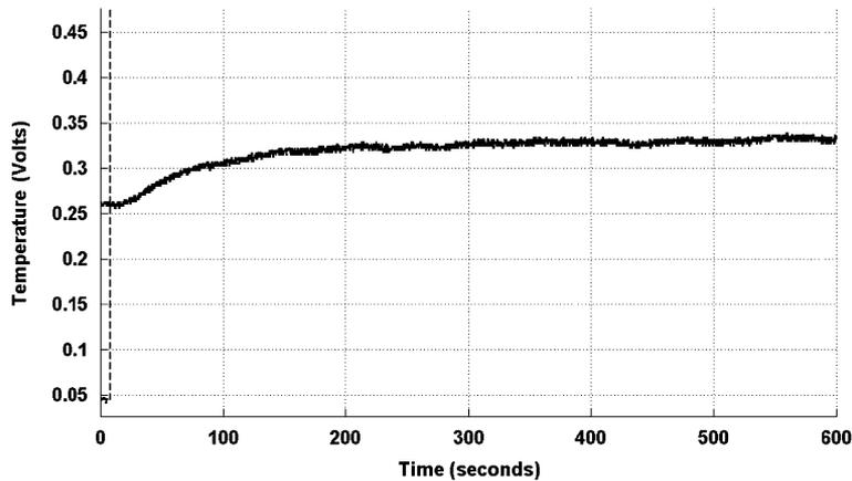
Figure 2. Step response of the process.
