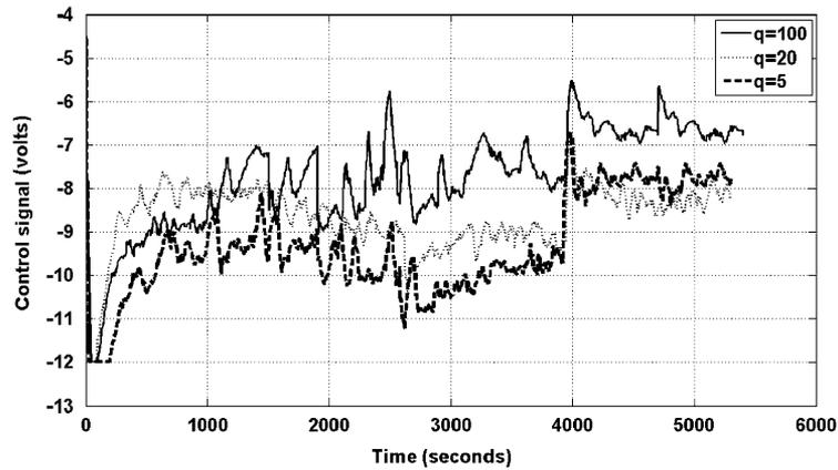
Figure 17. Implemented optimal control signals with the composed Trapezoidal rule.
