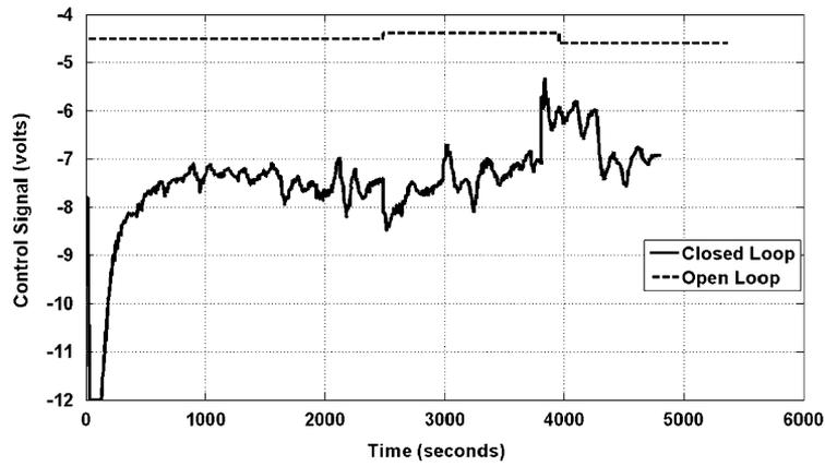
Figure 10. Control signals in open and closed loop.
