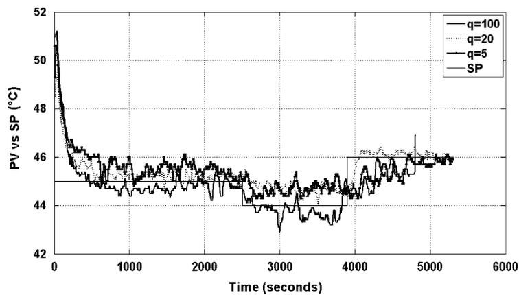
Figure 11. Comparison of PV responses with optimal control law approximated by composed Simpson's rule.
