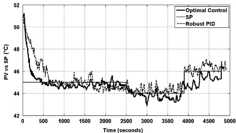
Figure 13. PV versus SP with optimal control and robust PID.
