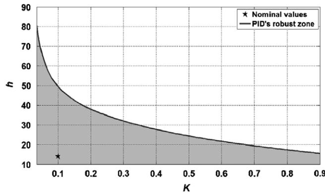
Figure 15. Robust stability zone for the PID controller.
