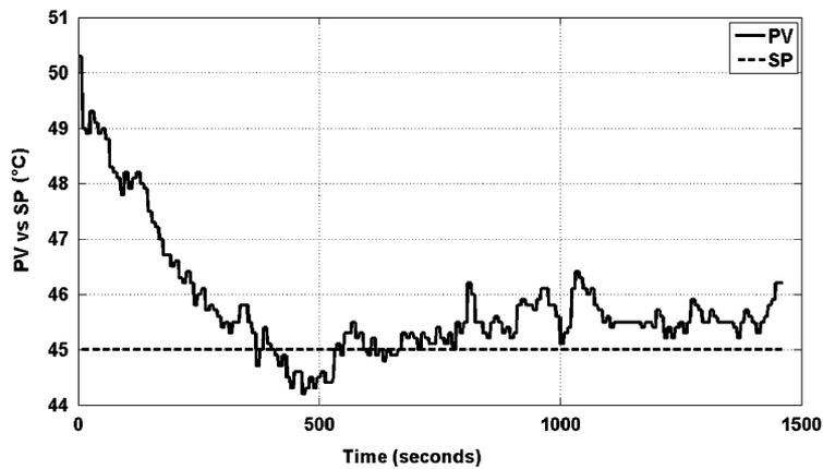
Figure 7. PV versus SP under disturbances when the gain is increased.
