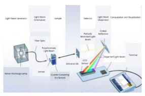
Figure 1. Operation of the Spectrophotometer.15
