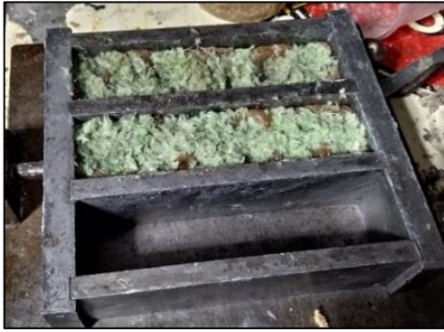
Figure 2: Mixtures of polyester resin, silica sand and PET fibers.
