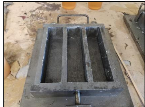
Figure 1: Steel mold for specimen preparation.
