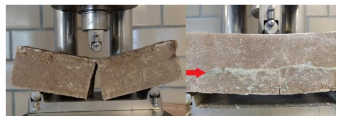
Figure 4: Control specimens (a), and concrete with PET fibers (b), after flexural tests.
