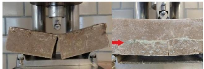
Figure 4: Control specimens (a), and concrete with PET fibers (b), after flexural tests.
