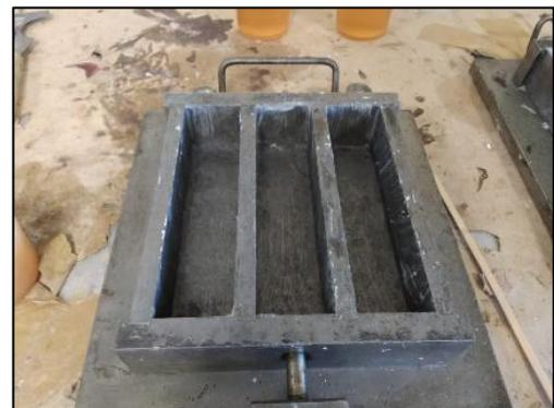
Figure 1: Steel mold for specimen preparation.
