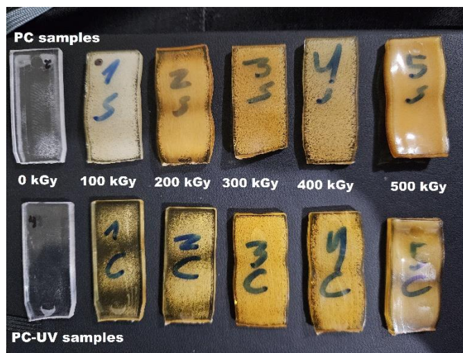
Figure 8: Below glass transition annealing results.
