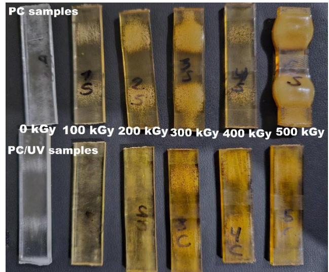
Figure 7: Post-DMA testing specimens
