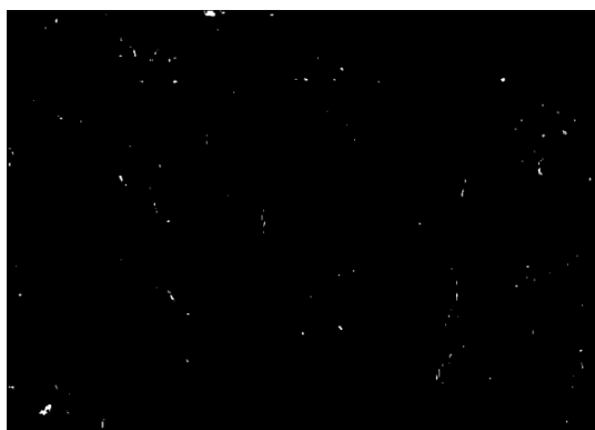
Figure 5. Processed microphotographs of the undamaged sample inside the SAE 1018 carbon steel pipe.
